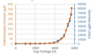
Figure 3: Field emission current and total light intensity vs. gap voltage from the measurement in Fig. 2 (c).
