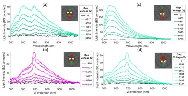
Figure 2: Spectra measurements from each perpendicular angle and both polarities. (a) Conditioning polarity transverse anode, (b) Negative polarity longitudinal anode minus noise, (c) Conditioning polarity longitudinal anode, (d) Negative polarity transverse anode.
