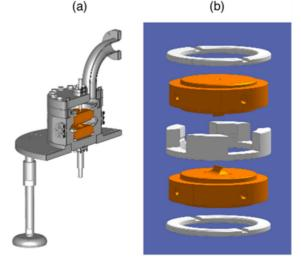
Figure 1: (a) CAD drawing of the LES vacuum chamber and (b) Exploded view of crossed ridged electrodes and ceramic spacers [10].
