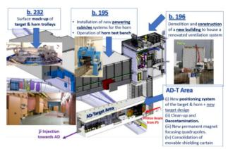
Figure 1: Scheme of the AD-Target area and related surface buildings involved in the consolidation activities.
