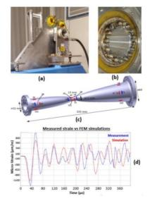
Figure 4: (a) Picture of a new horn in its test bench assembly. (b) Damaged horn during testing. (c) 3D model of the horn with the position of the optical strain gauges. (d) Measured dynamic response and simulation crosscheck.
