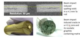
Figure 2: Images of a neutron tomography of in-beam tested Ta cores. Pictures of a fractured Ir core and graphite matrix after extraction from the prototypes tested in HRMT-48.
