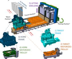
Figure 5: Sketch of the new trolleys system.
