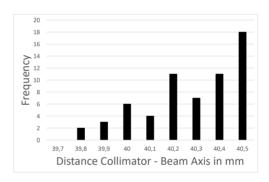
Figure 4: Frequency distribution of distances between beam axis and collimator block. It is specified to  $40 \pm 0.5$  mm.
