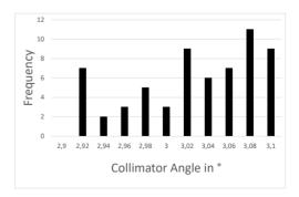
Figure 5: Frequency distribution of angles between beam axis and collimator block. The specification is  $3^{\circ} \pm 0.1^{\circ}$ .
