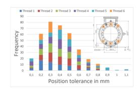
Figure 3: Achieved position tolerance of the six M10 thread holes for the fixation downstream. The specified tolerance is 0.5 mm.
