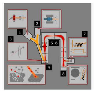
Figure 4: Schematic of a typical dynamic SIMS instrument: High energy (usually several keV) ions are supplied by an ion gun (1 or 2) and focused on to the target sample (3), which ionizes and sputters some atoms off the surface (4). These secondary ions are then collected by ion lenses (5) and filtered according to atomic mass (6), then projected onto an electron multiplier (7, top), Faraday cup (7, bottom), or CCD screen (8).
