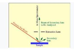
Figure 3: Schematic of SIMS.
