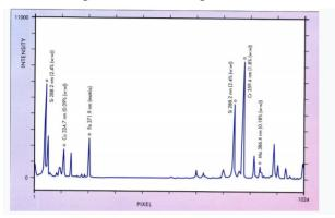
Figure 2: An example of a spectrally segmented emission spectrum of glow discharge using a Grimm-type glow discharge lamp with floating restrictor (8-mm diameter): 50 mA, 3.5 Torr, 2 kV; 22 Plasma array spectrometer (LECO); steel sample: 217A (Research Institute, CKD, Prague).
