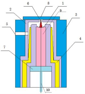
Figure 5: The scheme of the discharge device with self-focusing ion beam. 1- anode; 2- cathode; 3- case; 4- insulator; 5-gas supply; 6-focused ion beam; 7-window; 8-sample, 9-discharge plasma, 10-fiberglas optic.
