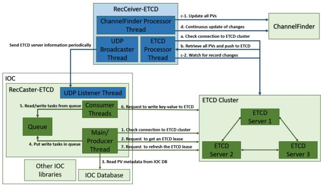
Figure 2: Schematic diagram of RecSync-ETCD operation with ChannelFinder. The work described in this paper is shown as the blue-colored. The operation orders of RecCeiver-ETCD and RecCaster-ETCD are labeled as  $1 \sim 7$  and  $a \sim d$ , respectively. Note that c-1 and c-2 run concurrently and the UDP Broadcaster Thread is atomic.
