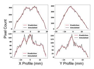
Figure 4: Predicted and simulated profiles for laser profiles withheld from training.
