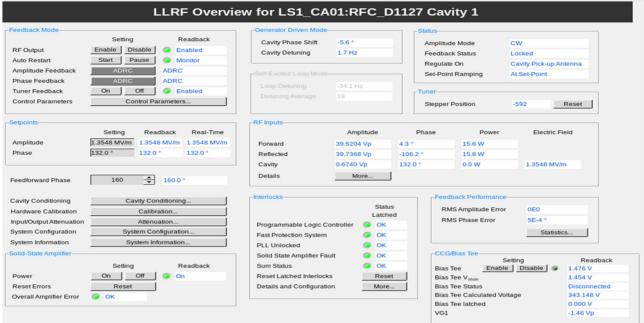
Figure 1: CS-Studio LLRF main OPI screen for a single cavity.
