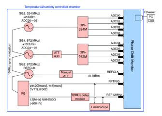
Figure 3: Schematic diagram of the PDM test setup. SG1&SG2, FG, DIV324M&DIV972M, and ATT indicate signal generators, function generator, 4-way dividers, and attenuator, respectively.
