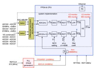
Figure 2: The functional block diagram of the PDM system. DDC, ROT, LPF, VS, and PS indicate digital down converter, IQ rotation, low-pass filter, vector sum, and processing system, respectively, whereas REFCLK, REF12MHz, RFTRIG, ADCLK, and FPGAREF indicate reference 972 MHz clock, reference 12 MHz signal, rf trigger, ADC clock, and FPGA reference clock, respectively.
