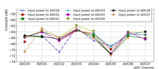
Figure 4: Crosstalk level in the PDM board. Note that the results for the ADC channels are displayed except for the channel in which rf power is applied.
