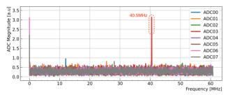
Figure 5: Crosstalk from REFCLK to the ADC channels.
