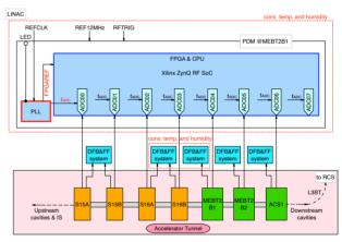
Figure 1: Block diagram of the phase drift compensation system to be implemented in linac.
