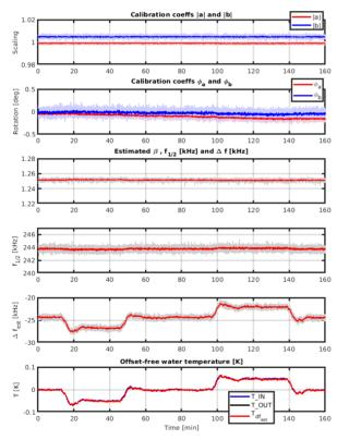
Figure 2: RF-gun temperature scan by changing the input water temperature by +0.05 K and keeping the drive amplitude constant. The online computed data is shown as light grey line and a moving average of 20 samples as blue and red lines for the upper plots. The last plot shows the comparison of the measured water temperature with update rate of 1 Hz and the estimated RF-gun temperature with moving average of 20 samples at 3.33 Hz to 5 Hz.
