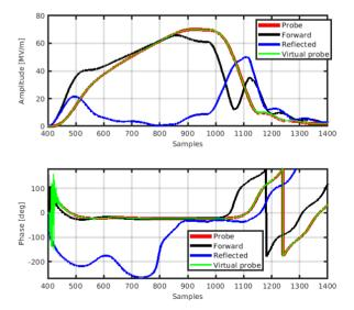
Figure 1: Calibrated signals of the ARES RF-gun in amplitude and phase for the probe, forward and reflected signal together with the virtual probe.
