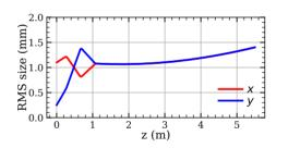
Figure 4: Backward tracking of the electron bunch starting from the undulator entrance (z = 0).
