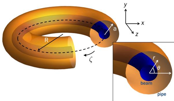
Figure 1: Unbunched beam in a toroidal conducting pipe, showing the coordinate system Eq. (1). The direction of beam current (inset) is out of the page. The bending is due to an applied uniform vertical magnetic field  $B_{bend}$ .
