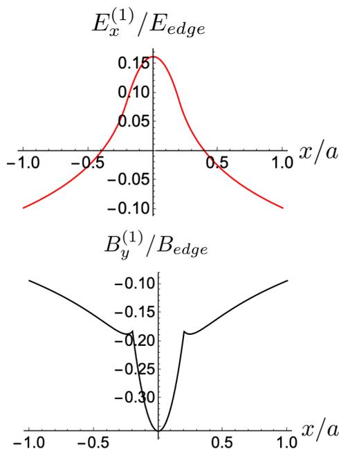
Figure 3: First-order curvature correction Eq. (16) to the space charge fields of a long uniform beam for the case  $b/a = 1/5$ . The beam edge is located at  $x/a = \pm 1/5$ .
