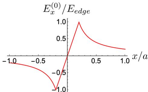
Figure 2: Space charge fields Eq. (14) for a long uniform beam in the zero-curvature limit for  $b/a = 1/5$ , shown in the bending plane in coordinates Eq. (15). The behavior of  $B_y^{(0)}/B_{edge}$  is identical.
