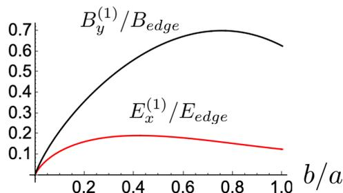
Figure 4: First-order curvature correction at the center of the beam as a function of the ratio  $b/a$ .
