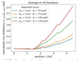
(b) Random tilt angles with respect to the optical axis. Figure 4: Emittance growth induced by randomly misaligned sections, for differing alignment errors  $\sigma_{\Delta x}$  and  $\sigma_{\delta}$ .
