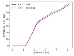
Figure 3: Center of mass transverse displacement induced by a misaligned section ( $\Delta x_2 = 50 \, \mu m$ ,  $\delta_2 = 50 \, \mu rad$ ).
