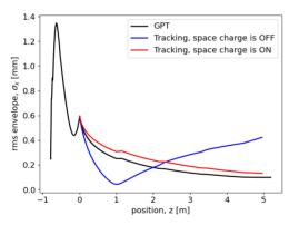
Figure 1: The effect of transverse space charge forces. Injection in the 4 section linac occurs at z = 0.
