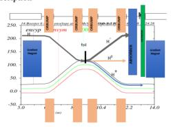
Figure 1: Schematic of the PIP-II Booster injection region. The H<sup>-</sup> ions are injected vertically. The vertical orbit is deflected using four orbumps magnets and the beam hits the foil at a fixed location near the inner lower corner of the foil.
