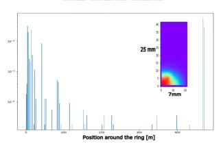
Figure 5: Large angle loss pattern. Losses around 470 m (upstream of the injection point) are likely due to a reduction in available vertical aperture at that location.
