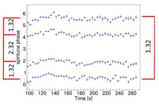
Figure 4: Relative horizontal polarization phase in radians of the four beam bunches as seen at the polarimeter (see text).
