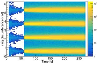
Figure 2: Detector rate as function of time within a beam store (x-axis) and position in the ring (y-axis), depicting the well separated four bunches. After beam cooling, the data acquisition starts at 60 s.
