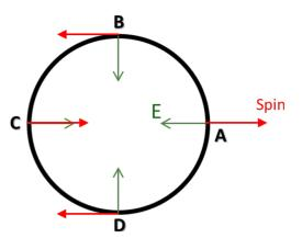
Figure 3: An illustration of a top down view of the ring at a fixed time with four bunches. The arrows show the particle-frame electric field (green) and the polarization direction (red). This pattern allows the search to be sensitive to to all phases.
