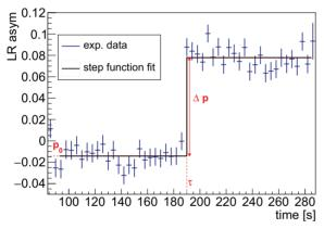
Figure 6: Polarization jump seen at resonance crossing in the case of the RF Wien filter scan. Also shown is the step function fit used to calculate the jump magnitude at resonance crossing.
