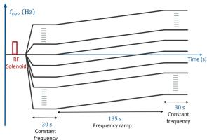
Figure 5: Schematic diagram of the scanning process (see text). The horizontal axis is time and vertical axis is the revolution frequency of the machine. The red rectangle marks the time of the RF solenoid operation.
