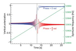
Figure 1: Example calculation where the spin precession frequency (green) was varied in search of a resonance. The signal is the jump in the vertical polarization at resonance crossing. The blue and red curves show calculations done at phases of 0 rad and  $\pi/2$  rad.
