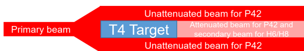
Figure 2: Schematic side view of proton beam being defocused before T4 target and partially interacting with it.
