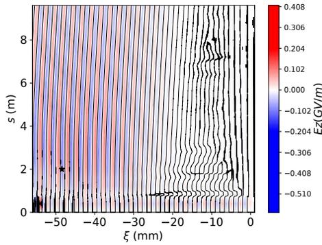
Figure 4: Evolution map of the on-axis longitudinal plasma wakefield  $E_z$  for the uniform plasma profile case. The black star marks the position where the maximum accelerating gradient is measured.
