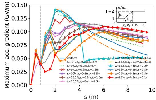
Figure 3: The maximum accelerating gradient for distinct plasma density profiles. The vertical dashed line marks  $s = 0.8$  m. The insert at the upper-right corner shows the schematic layout of the plasma density step.
