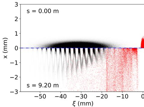
Figure 2: Simulation-obtained proton density (black) and electron macroparticle (red) distribution plot at the beginning (up-half,  $s = 0$  m) and after self-modulation (down-half,  $s = 9.2$  m). Longitudinal plasma profile: Uniform.
