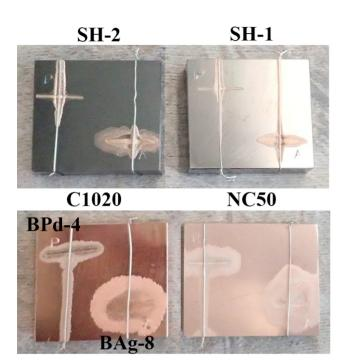
Figure 3: Results of brazing test.
