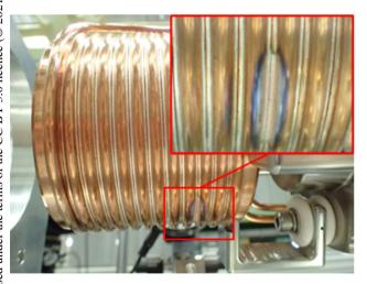
Figure 1: Typical discharge mark.
