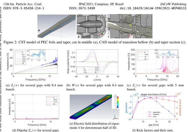
Figure 3: Simulation results for CPMU17.
