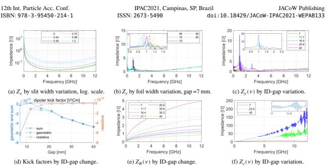
Figure 5: IVUE32 impedance spectra and kick factors by variation of different parameters.
