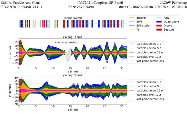
Figure 3: Losses along ThomX. The upper part represent the ThomX line from the TL to the end of the first ring turn. The lower part is plots of tracking of particles in x (at the middle) and y (at the bottom) plan along the accelerator.
