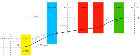
Figure 1: Sketch of the injection of ThomX. STR mean steerer, DPI mean injection dipole, BPM mean Beam Position Monitor, QP mean quadrupole.
