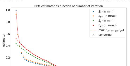
Figure 3: Evolution of the estimator at each iteration of the injection feedback code. The percentage of correction applied at each step depends on the maximum differences between each used and computed deviations  $\delta C$  as follows:  $\delta C > 1 \times 10^{-4} \rightarrow 10\%$ ,  $\delta C > 1 \times 10^{-5} \rightarrow 20\%$ ,  $\delta C < 1 \times 10^{-5} \rightarrow 100\%$ .
