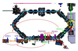
Figure 2: Overview of the ThomX's ring with localisation of the elements used in the injection feedback code.
