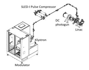
Figure 3: High Power RF Network.
