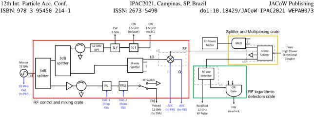
Figure 1: Simplified diagram of the Low Level RF System layout. The three coloured boxes define the three crates. Blue arrows define signals which are sent to the PXI control system.
