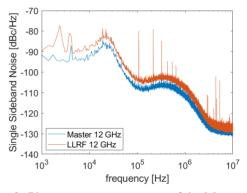
Figure 2: Phase noise measurement of the Master 12 GHz ((a) in Fig. 1) and the output of the LLRF ((b) in Fig. 1).
