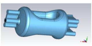
Figure 2: Vacuum volume of the EIC crab cavity.
