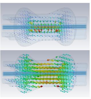
Figure 3: Electric (top) and Magnetic (bottom) field of the crab cavity.
