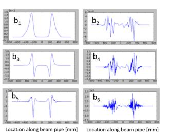
Figure 4: Normal multipole strength  $b_n$  along beam axis. The vertical axis of each plot has the unit of mTm/m<sup>n-1</sup>.
