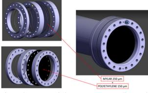
Figure 2: XCET window components: radiator tube, flanges, O-rings, and the two superimposed windows (on the inner part the Mylar window and on the outer, the black polyethylene window).
