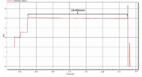
Figure 4: Pressure over time during pneumatic burst test. The spike around 2.25h shows the time when the pressure rose to failure reaching 6.5 bar before bursting.
