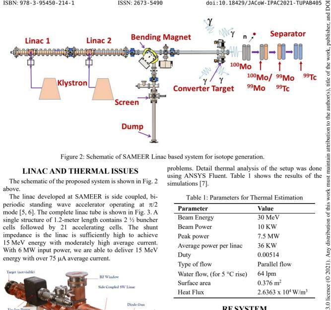
Figure 2: Schematic of SAMEER Linac based system for isotope generation.
