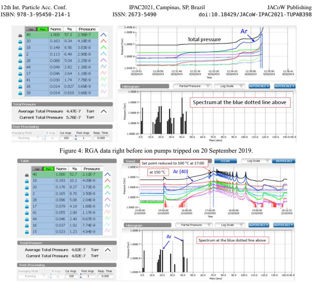
Figure 5: Detailed RGA data from 14:00 to 20:17 on 10 February 2020. At 15:00, something triggered the increased level of gas release and the pressure was going up fast. We decided to reduce the temperature to prevent RGA from tripping at 1E-5 Torr.
