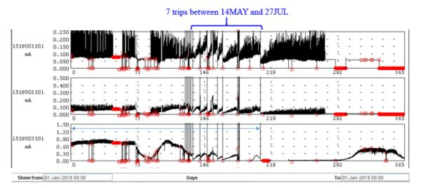
Figure 2: Ion pumps currents in 2018. A total of 7 trips occurred. The reason why there was no trip after 27 July 2018 is unknown.
