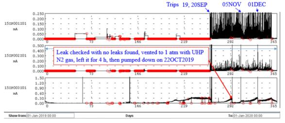
Figure 3: Ion pumps currents in 2019. A total of 4 trips occurred in 2019.
