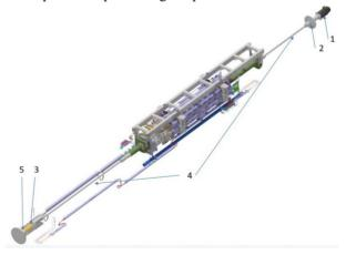
Figure 4: Measuring probe inside cryostat (not shown)1 – servo-motor; 2 - magnetic fluid rotary feedthrough; 3 slip-rings; 4 – stainless steel tubular shafts with two bellows compensators; 5 – angular encoder.
