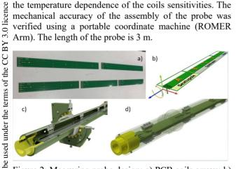
Figure 2: Measuring probe design: a) PCB coils arrays; b) boards arrangement inside unit; c) and d) internal design pf the probe.
