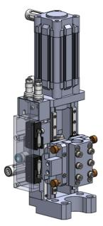
Figure 6: The picture of Photon shutter.
