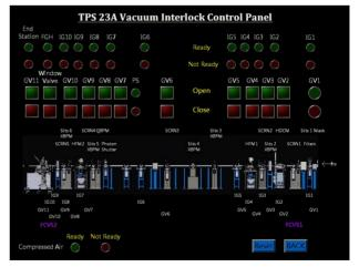
Figure 7: The picture of Vacuum Interlock Control Panel.
