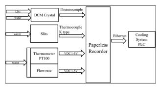
Figure 9: System architecture of Cooling System.
