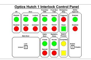
Figure 3: The picture of Optics Hutch Interlock Control Panel.
