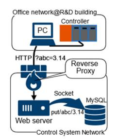
Figure 3: System chart of sending archiving data from the R&D building to MyDAQ2 through a reverse proxy.
