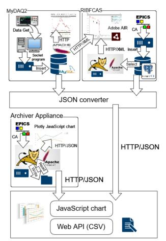
Figure 1: System chart of linkage methods with existing systems. The clients obtain the archived data through the JavaScript chart or Web API.
