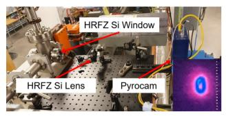
Figure 4: HRFZ Si system at the MAX IV SPF. Inset image is the first test image of CTR with the system.
