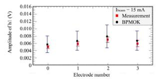
Figure 3: Comparison of predicted first harmonics from BPMOK and the measurement for each electrodes of the BPM. The error bars represent uncertainties at 2 RMS.
