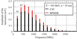
Figure 6: BPMOK vs CST: DFT of typical output signal from the BPM with a 50 mm radius for a centred beam.
