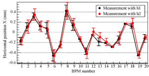
Figure 4: Measured horizontal position of the beam in the LINAC of SPIRAL2 as a function of the BPM number.
