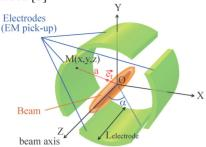
Figure 1: Scheme of the BPM and the position of the point M on the electrode's surface where the field induced by the beam is integrated.
