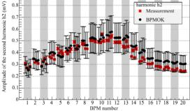
Figure 5: Variation of h1 and h2 amplitudes along the LINAC as a function of the BPM number. The measurements and the predictions of the model BPMOK are compared. The error bars represent uncertainties at 2 RMS.
