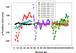
Figure 5: Examples of the variation of the beam vertical centroids bunch by bunch for 50 m icropulses at B102, B120, and B121 for V103 settings of +2.0,-1.5, and 0.0 A from the reference. These were 100-shot averages to show the  $\sim$ 220-kHz oscillation effects generated in CC2 [11].
