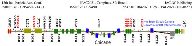
Figure 1: Schematic of the FAST beamline layout showing the PC rf gun, capture cavities (CCn), correctors (H/Vnnn), rf BPMs (Bnnn), chicane, OTR and YAG:Ce screens (Xnnn), the spectrometer dipole bend magnet (D122), and the beginning of the cryomodule (CM).
