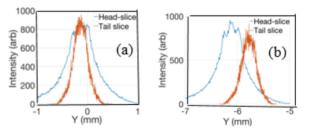
Figure 6: ASTRA simulation results of the head-tail kick for (a) no y offset with no y-t kick and (b) 5-mm y offset through the cavities with a calculated  $\sim$ 500-µm head-tail kick.
