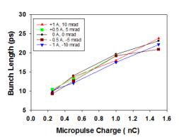
Figure 4: Streak camera bunch length versus charge results during a V101 corrector scan from -1.0- to +1.0-A values. At 4.5 MeV, a 1-A current change corresponds to a 10-mrad angular change into CC1. The transverse laser spot is  $\sim 0.5$  mm in x and y in this case [12].
