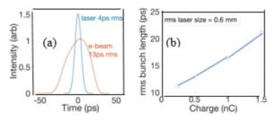
Figure 7: ASTRA simulation results for the electron-beam bunch length at (a) 500 pC/b compared to the initial laser pulse length and (b) as a function of charge from 0.25 to 1.5 nC.
