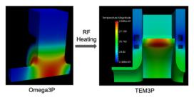
Figure 1: Temperature distribution in cavity enclosure due to rf fields of the cavity accelerating mode.
