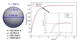
Figure 2: (Left) Simulation model and material properties; (Right) Maximum and minimum temperatures in sphere as a function of time, with insert showing agreement with analytical solution at a time step.
