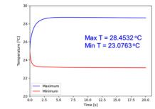
Figure 3: Evolution of minimum and maximum temperatures inside rf gun cavity.
