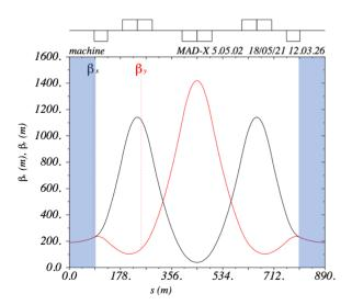
Figure 2: Beta functions of T-insert lattice designed for the IBEX trap. Blue shaded region is the drift region for the nonlinear insert.
