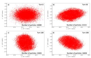
Figure 4: Phase space when a quadrupole perturbation is applied to the T-insert lattice, at a frequency of  $2 \cdot 2\pi Q$ , with the octupole potential switched on.
