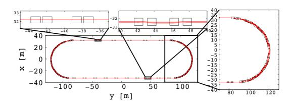
Figure 1: Schematic of the nuSTORM decay ring, designed in FixField, with normal quadrupoles (top straight part), circular scaling FFA (arc parts) and straight scaling FFA cells (bottom straight part).
