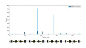
Figure 3: Beam loss distribution along the ring. The yellow box at the bottom represent the dipoles.
