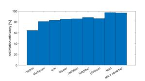
Figure 9: Collimation efficiency comparison from different materials.
