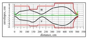
Figure 7: Horizontal (H) and vertical (V) <sup>197</sup>Au<sup>26+</sup> beam envelopes, aperture (red line) and longitudinal magnetic field (green line).
