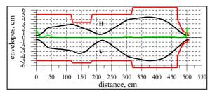
Figure 6: Horizontal (H) and vertical (V) <sup>209</sup>Bi<sup>38+</sup> beam envelopes, aperture (red line) and longitudinal magnetic field (green line).
