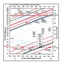
Figure 1: Working diagram of DC140 cyclotron.
