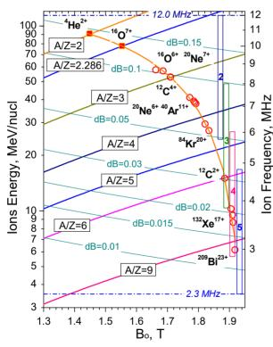
Figure 1: The operation modes diagram of U400M.
