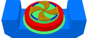
Figure 5: Computer model of U400M magnet with additional valley shims and machining of sector shims.
