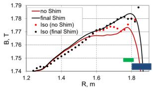
Figure 8: Magnetic field with and without final shimming, are shown by lines. Circles represent corresponding isochronous fields. Green and blue rectangles show sector and valley shims radial position.
