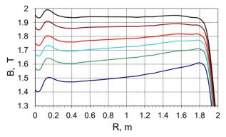
Figure 4: U400M magnetic field at operative levels.
