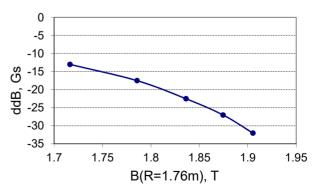
Figure 2: The change of magnetic field radial growth because of main coil reconstruction.
