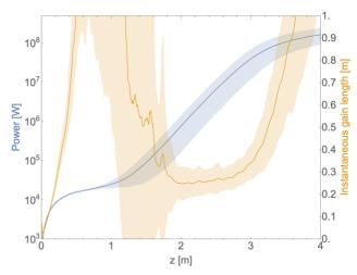
Figure 2: Plots showing the peak power (blue) and instantaneous gain length (orange) for GENESIS simulations of the EUV FEL detailed in Table 1. The shaded area corresponds to one standard deviation based on 16 SASE averaged runs. The large variation in shot-to-shot power is due to the high degree of slippage causing it to operate near single-spike mode.
