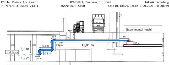
Figure 1: Beamline setup (not on scale). Light propagation is represented from the undulator source to the laboratory. M1 is plane OTR screen, M2 is an off axis parabolic mirror that collimates the beam to a plane mirror (M3). The radiation is focused by M4 into a long conduct where in the center is placed the diagnostic setup. M5, a parabolic mirror identical to M4, collimates the beam directing it to the experimental room.
