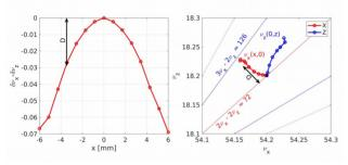
Figure 3: Left: dissonance along horizontal direction, right: on-momentum tune expansion.
