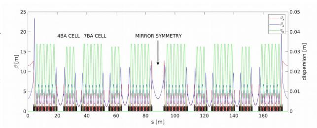
Figure 1: Super cell optical functions of the 7BA-4BA SOLEIL upgrade lattice producing an emittance of 80 pm mrad.
