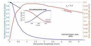
Figure 4: Coupling and vertical transfer versus horizontal initial amplitude at injection center.
