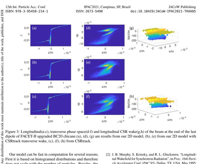
Figure 3: Longitudinal(a-c), transverse phase space(d-f) and longitudinal CSR wake(g,h) of the beam at the end of the last dipole of FACET-II upgraded BC20 chicane.(a), (d), (g) are results from our 2D model, (b), (e) from our 2D model with CSRtrack transverse wake, (c), (f), (h) from CSRtrack.
