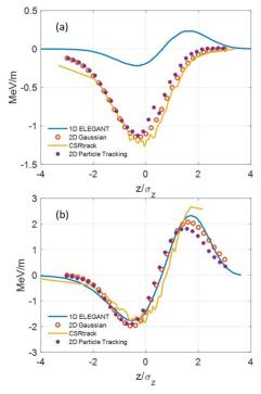
Figure 1: Longitudinal CSR wake along the central axis of the beam in the middle of the third (a) and fourth (b) bend of the benchmark chicane.
