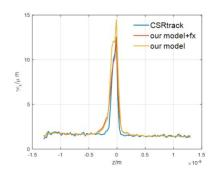
Figure 2: Slice emittance at the end of the last dipole of FACET-II upgraded BC20 compressor from CSRtrack(blue), our 2D model(yellow) and our 2D model with transverce force from CSRtrack(red).
