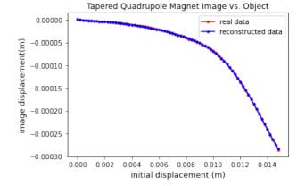
Figure 3: Image Displacement vs. Initial Displacement for the Tapered Quadrupole Magnet. The real data is exported from CST Studio particle tracking simulation and the reconstructed data is generated from the curve fit (polyfit).
