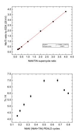
Figure 1: Linear relationship between the ratio of Nb to Ti concentration measured by EDX and the NbN to TiN ratio within the supercycle of PEALD (top) and variation of the critical temperature for the different ratios of NbN to TiN supercycles during the PEALD process (bottom).
