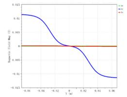
Figure 1: The field distribution of the nonlinear magnet adjusting the horizontal beam distribution.
