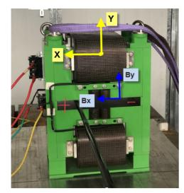
Figure 2: Nonlinear magnet adjusting the horizontal beam distribution.
