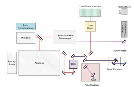
Figure 1: Schematic of SXFEL drive laser system.
