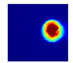
Figure 3: Laser spot image on virtual cathode.
