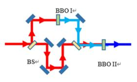
Figure 2: Schematic of the THG.
