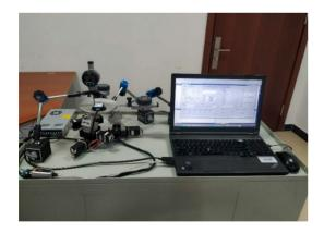
Figure 6: Positioning accuracy test of 6-DOF Platform.
