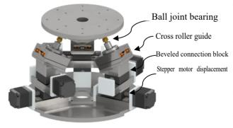
Figure 2: 6-DOF Platform driven by stepping motor.
