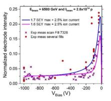
Figure 4: Variation of  $I_+/I_{electrons}$  vs V<sub>bias</sub>: experimental data (red circle recorded during different fills and purple cross for a voltage bias scanning during the fill 7328) and calculated values for several SEY (color lines) considering an ion current of 2.5% of the total electron one.
