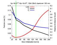
Figure 3: Loss and emittance growth as a function of the slow initialization time  $T_{init}$ .
