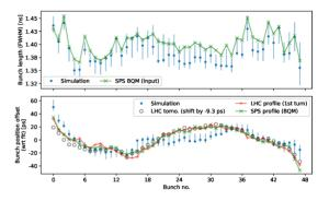
Figure 2: Bunch phase (position) offsets  $\Delta \phi_{bb}$  of the simulated (blue) beam reproducing a 48-bunch batch ( $N_b = 1.1 \times 10^{11}$  ppb ave.,  $\tau = 1.36$  ns ave.) in Fill 7137 generated in SPS at flat-top w.r.t. measurements (red, green, circles).
