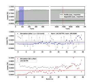
Figure 4: Injection losses from the SPS beam in Fig. 2 into the LHC.
