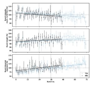
Figure 3: Average bunch-by-bunch intensity, bunch length, and binomial exponent relative to their batch-average for 48b batches from several 2018 fills, and model extrapolation to 72b batches.
