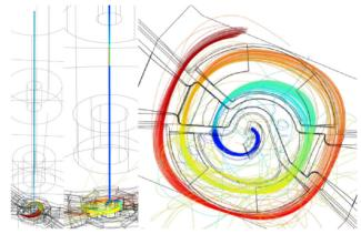
Figure 3: Continuous beam dynamics. Left – the main magnetic field calculated in COMSOL component; Center and Right – the main magnetic field imported from CST; Right – the inflector geometry is improved.
